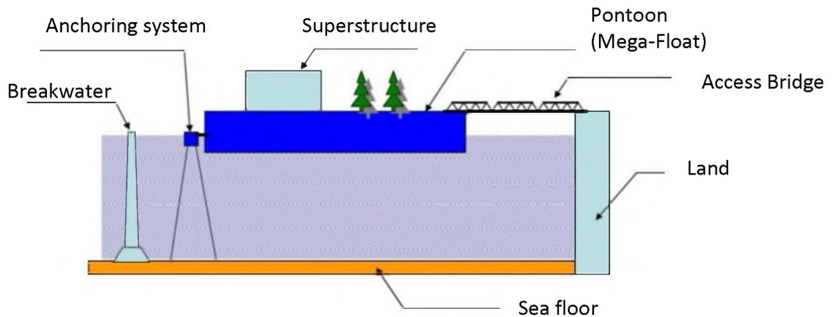
Figure 109: Mega-float: schematic arrangement of elements (49).
