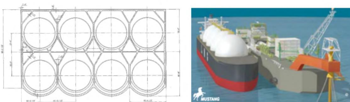
Figure 150: LNG FPSO concept of concrete hull Mustang: cross section and rendering (72).
