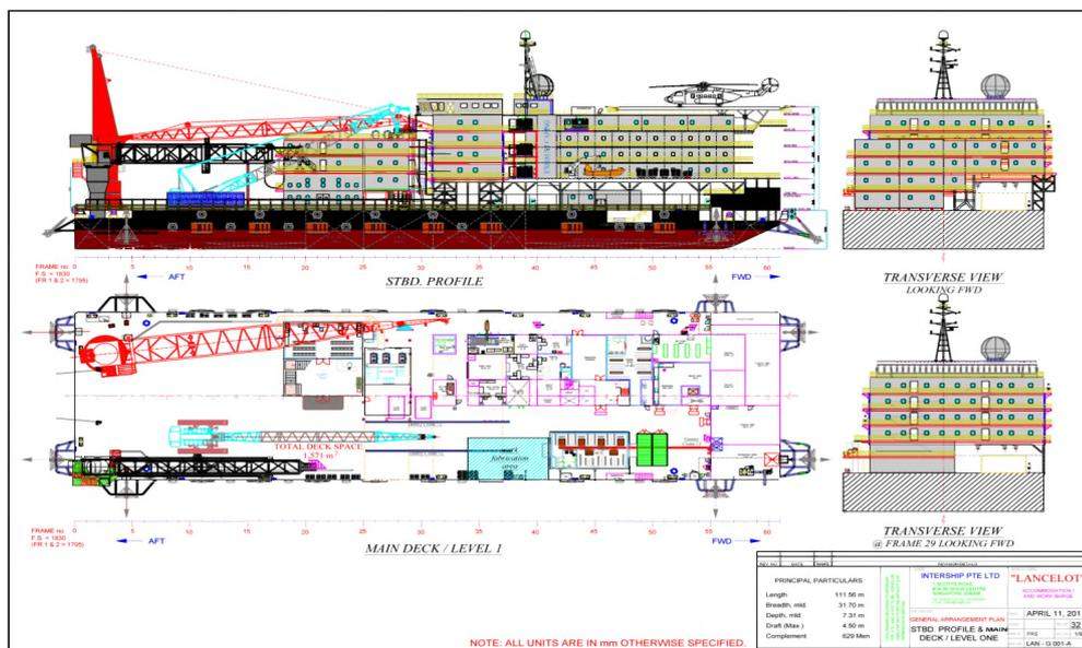
Figure 94: AWB Lancelot. Elevation, plan and sections.
