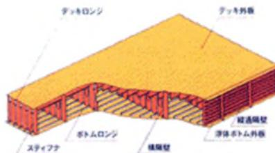
Figure 110: Mega-float: structural design of the pontoon (50).
