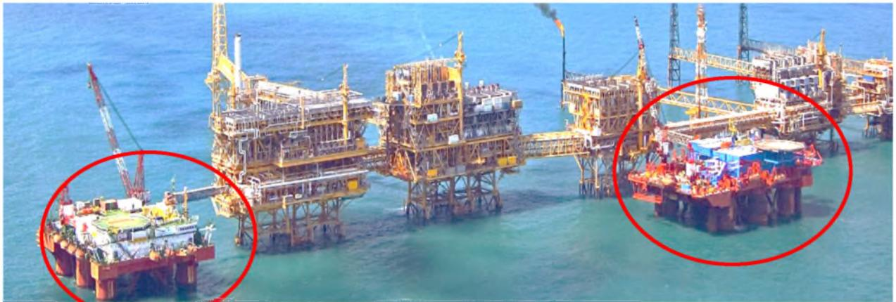
**Figure 80: Semisubmersible offshore flotel servicing an offshore oil field**
