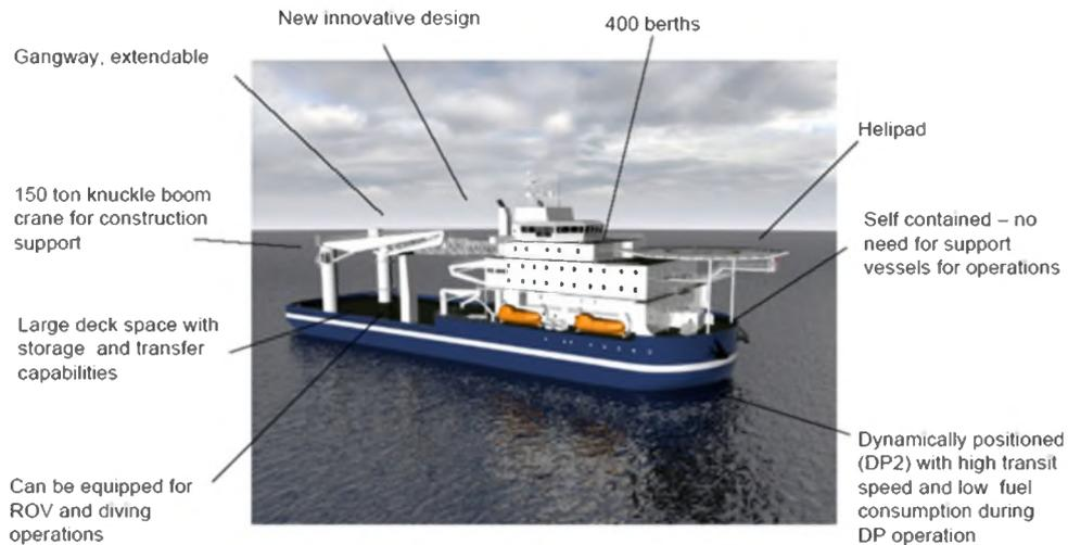
Figure 86: Layout of the flotel Ocean Hotels Plc
