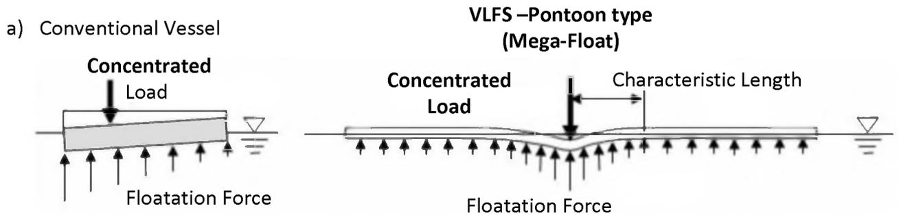
Figure 114: Overall response time under a static concentrated load (46)
