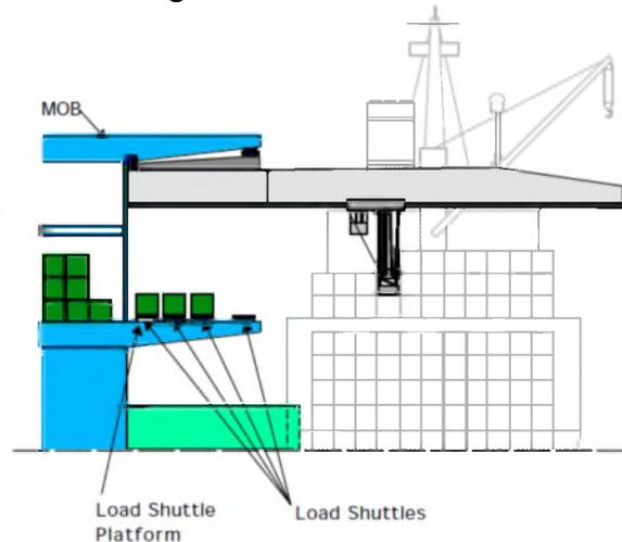
Figure 125: Load Transfer System (LO/LO) between an MOB and a ship (67)
