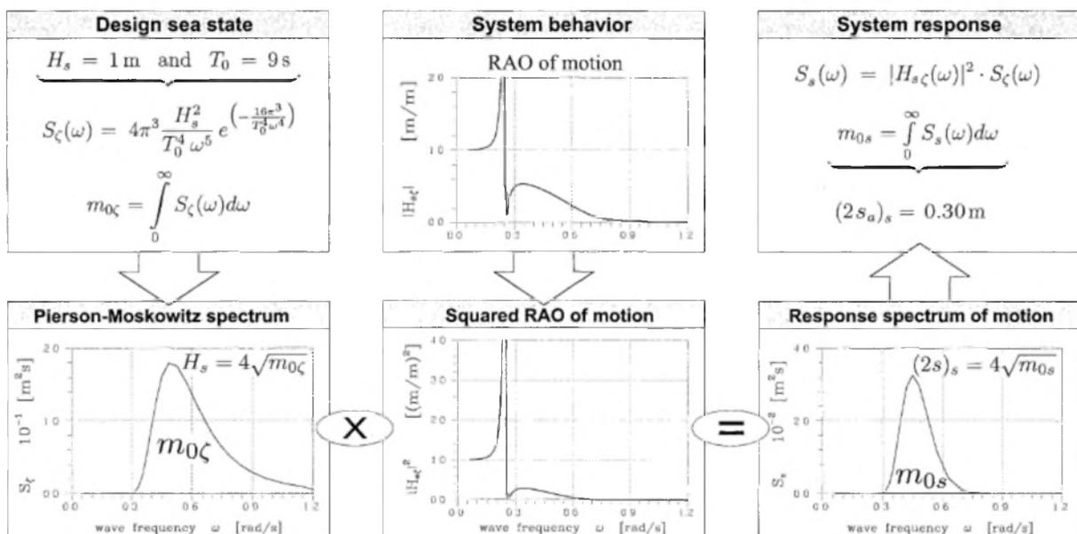
**Figure 180: RAO filters the wave signal spectrum (wave spectrum) to obtain the range of movements (*spectrum of motion*).**
