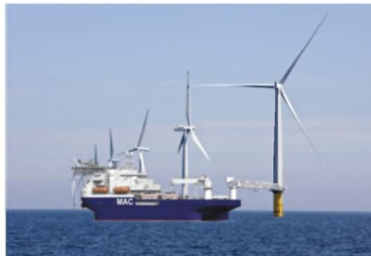
Figure 161: CSS-Seabreeze DP-3 Wind Farm Mother Ship. Source: MAC offshore.
