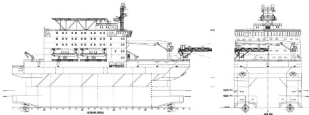
Figure 104: CSS Accommodator, profile and section
