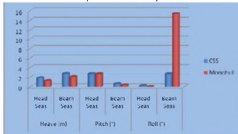
Graph 7: Comparison of behavioral characteristics in the sea with a single-hull 120m CSS.
