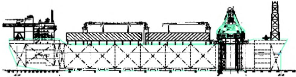
Figure 155: FPSO version with anchorage (Aalbers, Vries, & Vugt, 2006)
