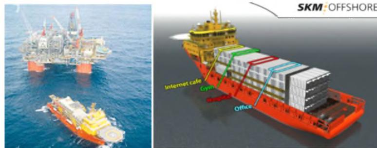
**Figure 84: Edda Fjord in operation as a flotel and a rendition with accommodation modules type container**
