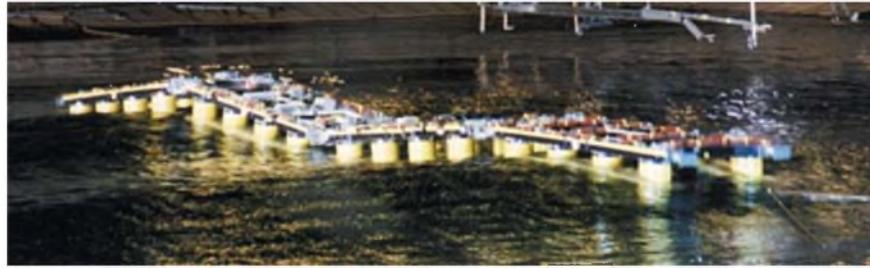
Figure 124: Tests to evaluate hydroelastic connectors (59)
