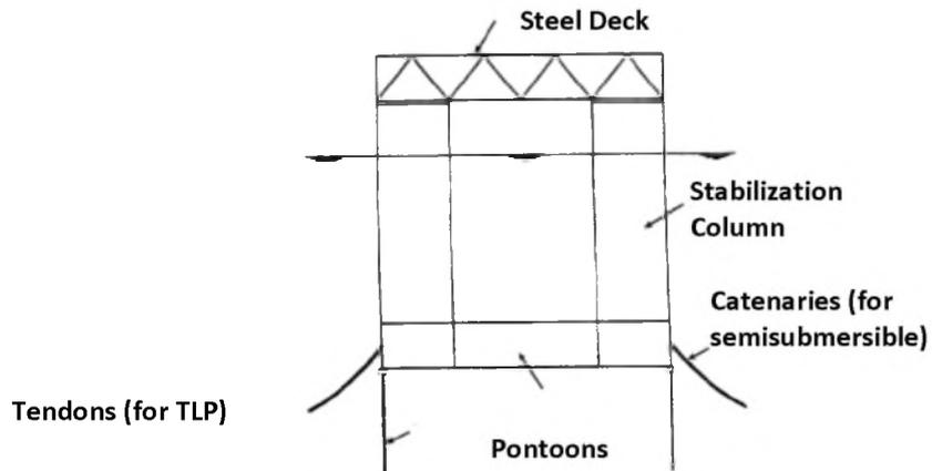
**Figure 143: Common semi-submersible platform and TLP diagram**
