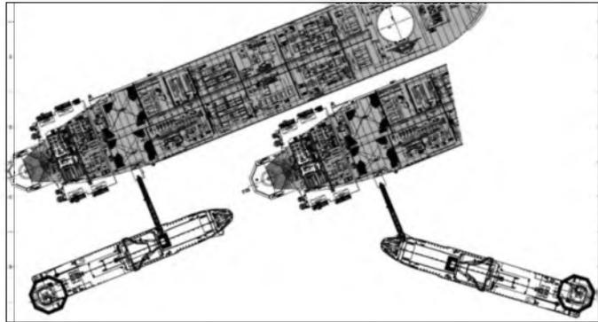
**Figure 89: System Access between the offshore accommodation ship and the FPSO Dan Swift.**
