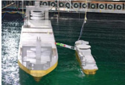
**Figure 186: Channel testing of the Accommodation Vessel model *Dan Swift*. Source: Offshore Lauritzen A / S**
