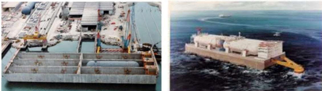
Figure 147: Floating LPG terminal "Ardjuna Sakti" (95)
