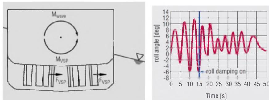
**Figure 92: Torque produced by the engines and their dampening effect on the rolling period (36).**
