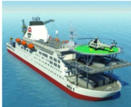
Figure 164: year 2015-2025: a cruise or ferry converted in Flotel
