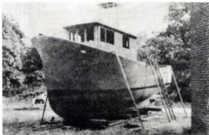
Atlantis II, the ferrocement ship built by Operation Atlantis, shortly before launching (from Atlantis News).
